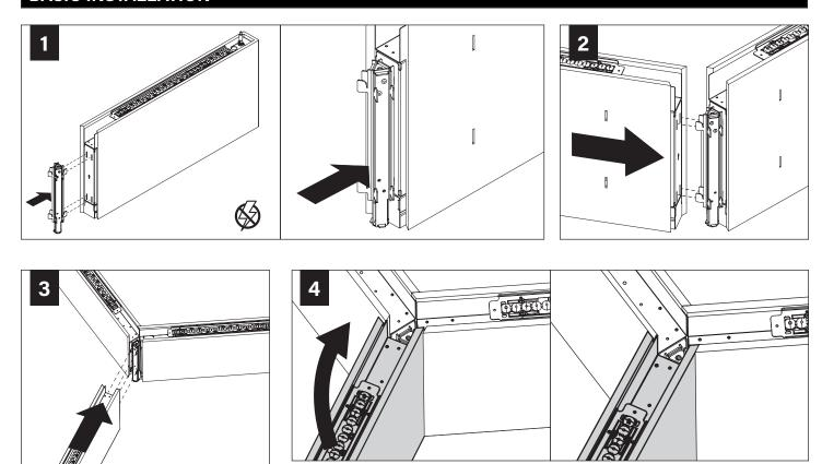
↑ SWING THIRD SECTION INTO PLACE SO IT INTERLOCKS WITH THE TWO OTHER SECTIONS
