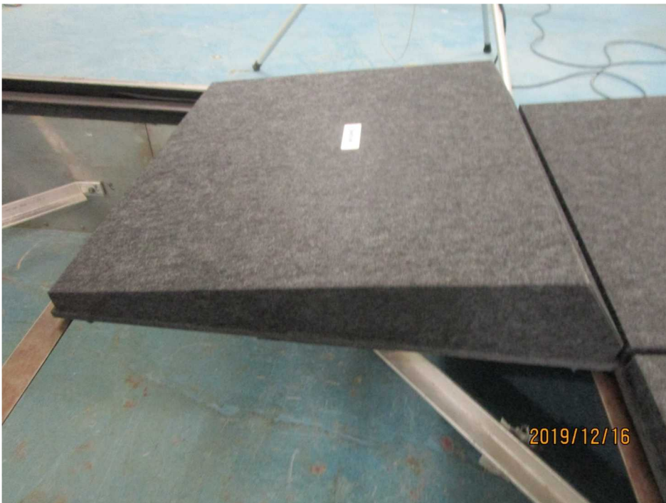
Figure 2 – Detail of individual tile, varying protrusion depth
