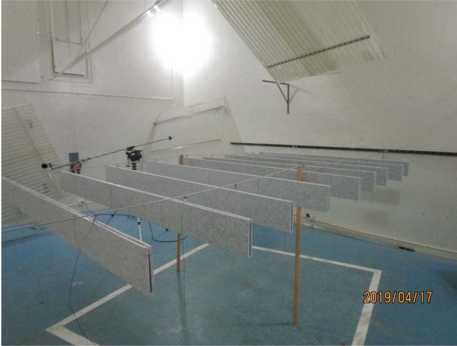
Figure 1 – Specimen mounted in test chamber
